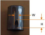
Each roller bearing was tested on both ends. For each test set there were 6 tests conducted. The measurements were taken using an 8:1 magnifying lamp and digital calipers. The width and height of each scar was measured and recorded. 5 out of the 6 tests per test set were used to determine the load bearing capability of the oil. The test outliner was removed from the calculation. The
