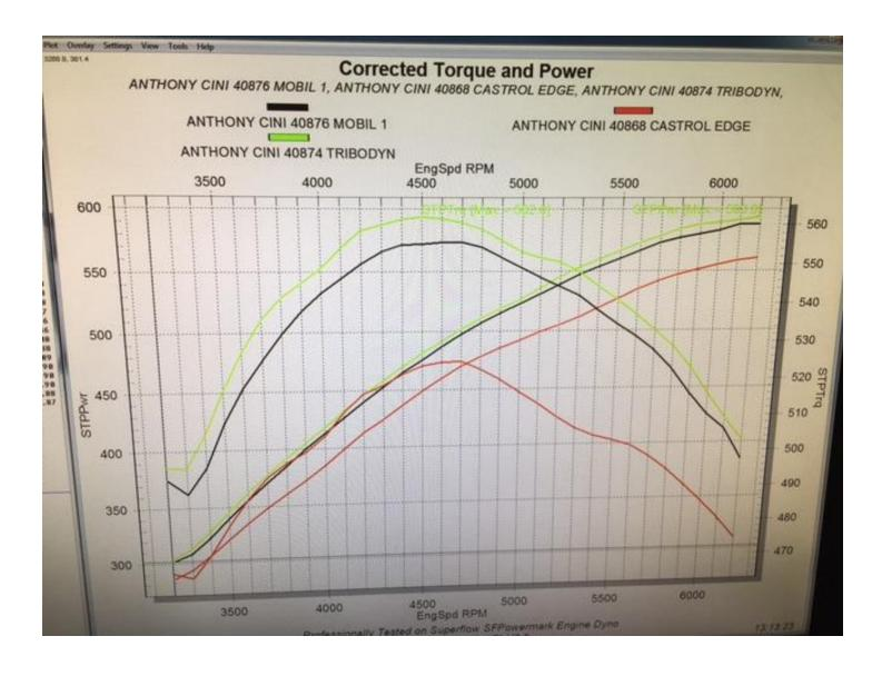
This Dyno test shows the maximum torque was 562 lb-ft and power was 590 hp. TriboDyn & Mobil 1 outperformed Castrol Edge by a substantial margin. TriboDyn exceed the 555 lb-ft and 582 hp of the Mobil 1 by 1.3% and 1.4% respectively.
